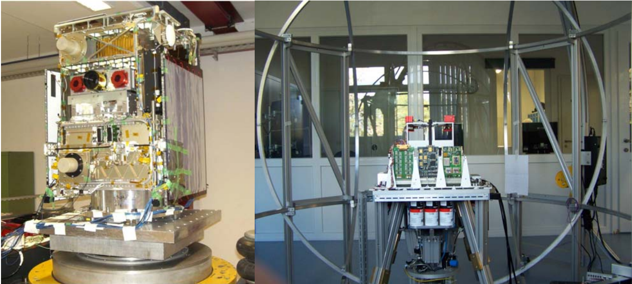
Fig. 9. STM on shaker (left), EM AOCS on test bed (right)
