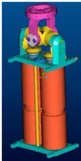
**Fig.2: Base joint unit and its actuation system**
