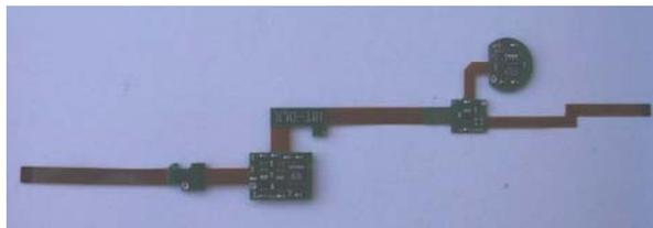
Fig.7 Flexible printed circuit board in the finger
