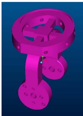
**Fig.4: Base joint torque sensor**
