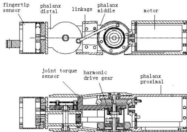
**Fig.3: Finger unit with one integrated actuator and two coupled joints.**
