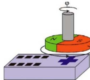
**Fig.5: Principle of measuring system by using integrated hall sensor**
