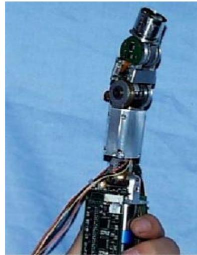
Fig.1: One finger of the HIT/DLR Hand
