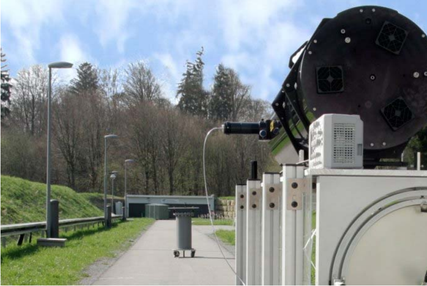
Laser based standoff detection at the free space optical test range.
