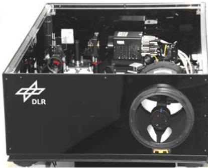
A mobile adaptive optics demonstration system used for high resolution imaging.
