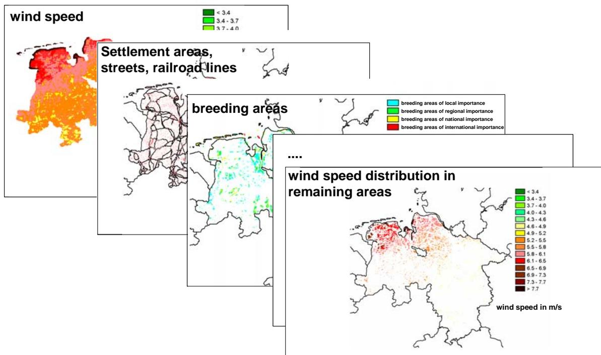
**Fig. 11: GIS-based estimate of wind energy potential subject to nature conservation restrictions, taking Lower Saxony as an example**
