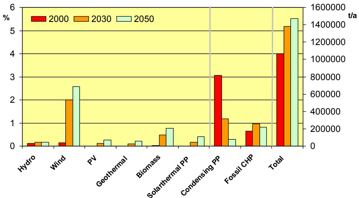
**Fig. 9:** Cumulative annual iron requirements for electricity generation in the “NatureConservationPlus” scenario, as a percentage of total iron demand in Germany in 2000 (without credits for CHP heat)
