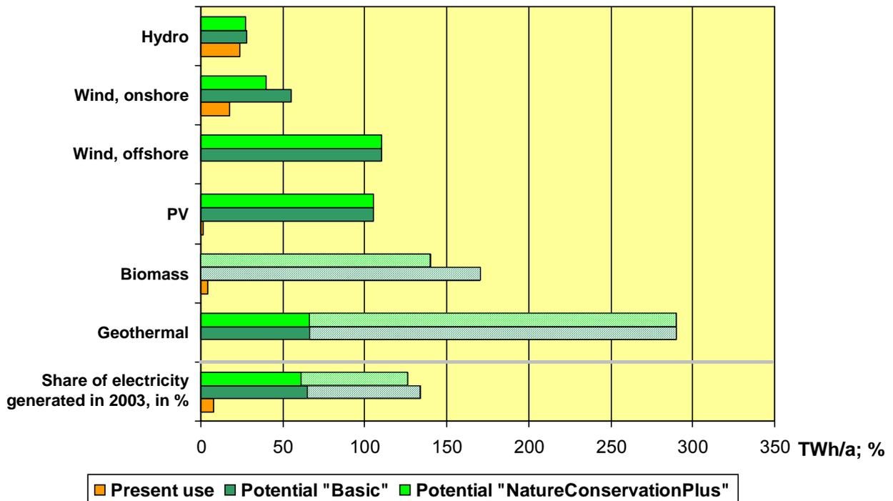
Fig. 14: Potential for electricity generation from renewable energy sources in Germany, excluding imports (hatched areas: potential subject to differences in biomass input options and other limitations)
