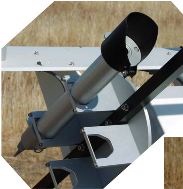
Figure 3: 'First class' Kipp&Zonen pyr heliometer for DNI measurement.
