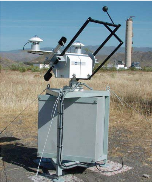
Figure 2: Meteo station with Kipp&Zonen pyranometer (GHI, DHI) and pyrhelimeter (DNI).
