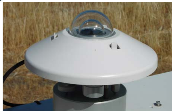
Figure 4: 'Secondary standard' Kipp&Zonen pyranometer for GHI and DHI measurement.
