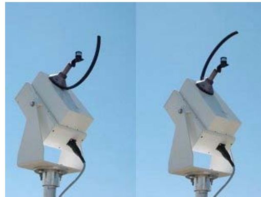
Figure 1: Rotating Shadowband Pyranometer (RSP) in normal position (left) and during rotation (right).
