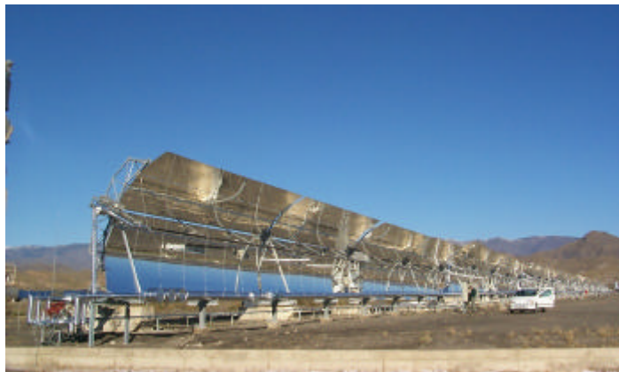
Fig. 7 The testloop of the European DISS project at the Plataforma Solar de Almería
