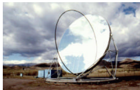
Fig. 10 The ASM-150; a 150m 2 stressed membrane heliostat
