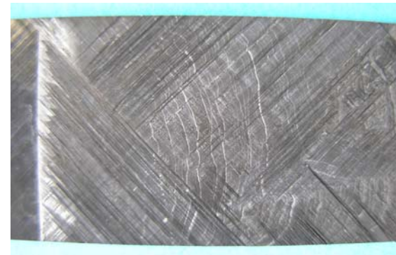
Curved crack front in 45° layup
