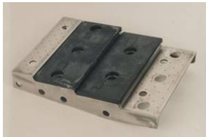
LuFo Brennkammer Schindeln MAN Tech. & DLR C/SiC
