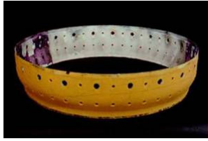
HTDU5 Brennkammerwand Dupont-Lanxide SiC/Al 2 O 3
