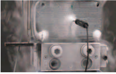
Testing setup for cryogenic tests at -196^{\circ}\text{C}
