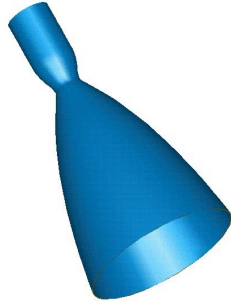
Figure 3 SE-12 Nozzle contour as generated by NCC
