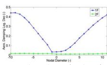
Fig. 4: Aerodynamic damping of tuned UHBR fan
