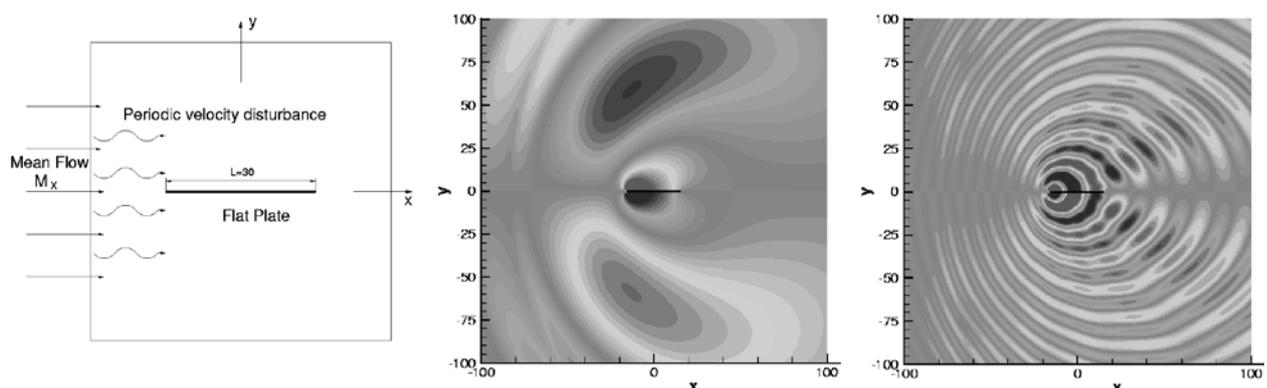
Sound generation at a flat plate due to incident gusts of different wave-lengths
