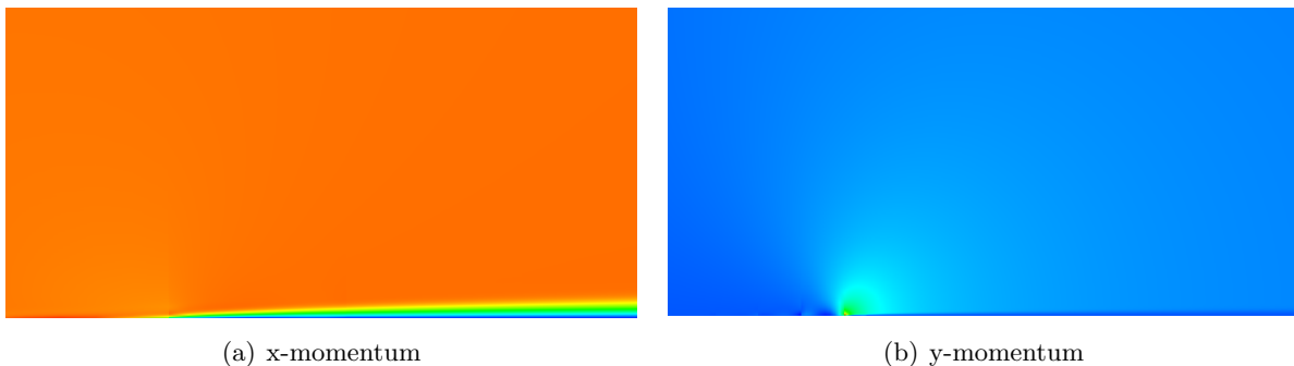
Figure 1: Momentum ( \rho u and \rho v ) contours near the plate.
