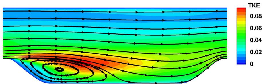
Figure 2: Streamtraces and turbulent kinetic energy computed on the time- and spanwise averaged velocity field. Simulation by 4<sup>th</sup> order Pade-scheme and 8<sup>th</sup> order implicit filter.
