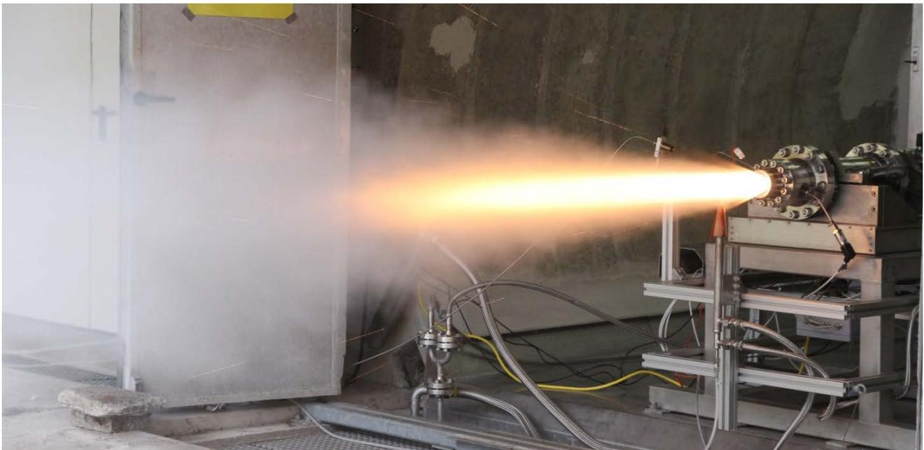
Experimental firing of the AHRES hybrid rocket engine demonstrator at the test bench at DLR Trauen
