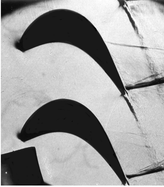
Figure 1: Schlieren photo of the 2-D flow field ( Ma_{2is} = 1.1 )
