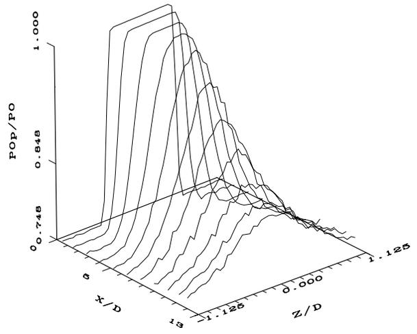
Figure 10: Total pressure of the free jet
