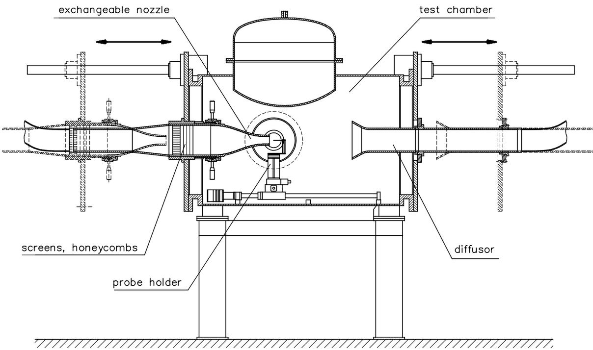
Figure 1: Test facility for probe calibration (SEG)
