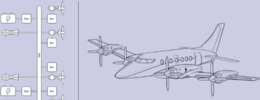
A completely battery-powered propulsion system is feasible for smaller, 19-seater aircraft for flights of up to 200 kilometres. Fuel would be carried only as a reserve in case of emergencies, or if the aircraft were required to fly longer routes.
