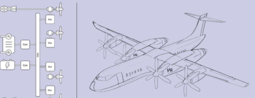
Medium-sized, short-haul aircraft flying up to 2000 kilometres could reduce CO<sub>2</sub> emissions through a clever combination of different propulsion systems. Hydrogen fuel cells power the aircraft during cruise and when taxiing on the ground. Batteries supply the on-board electrical systems. Hydrogen gas turbines provide the necessary thrust for take-off and potential go arounds.
