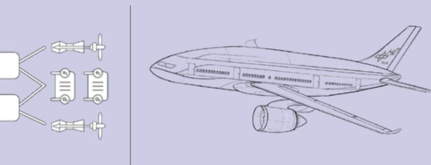
Larger aircraft carrying 150 passengers or more on medium-haul routes of over 2000 kilometres require greater propulsive power. Fuel cells are used when taxiing on the ground, while gas turbines that burn synthetic fuels allow for faster cruising flight. When used in parallel, both systems combined can generate enough power for take-off.
