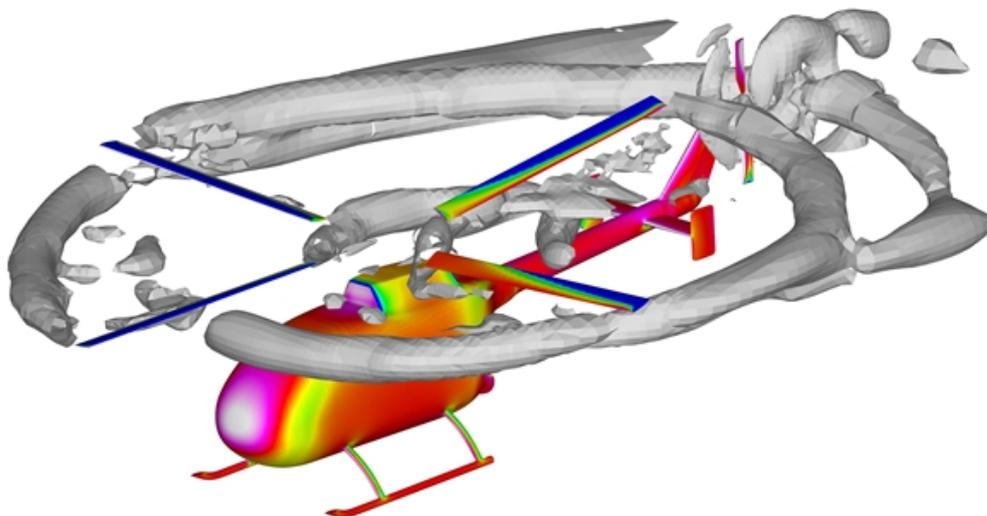
Reduced pressure on the top of the blade draws air upwards; this produces a vortex – the blade tip vortex – that is then directed downwards. When other rotor blades subsequently come into contact with these vortices, the 'chopping' or throbbing noise characteristic of helicopters is produced.
