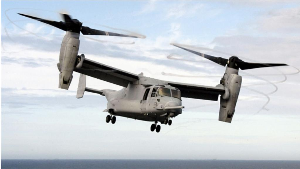
This image shows the vortices that form at the ends of rotor.
