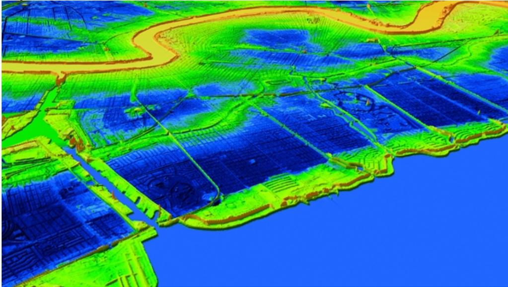
This coloured SRTM elevation model shows the elevations for New Orleans in the southern USA. Large parts of the city lie considerably below sea level and would flood without elaborate and extensive protective measures. The yellow and green zones lie above sea level, while the blue zones lie up to four metres below it.
