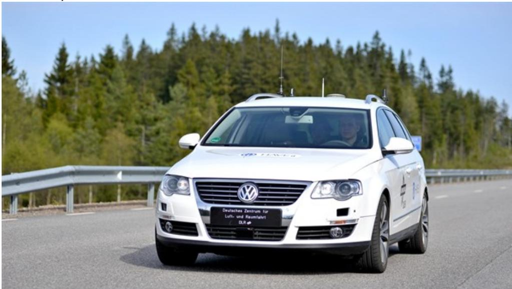
Equipped with sensors and an electronic steering system, steer-by-wire, the FASCar II is used to test innovative driver assistance and automation systems.
