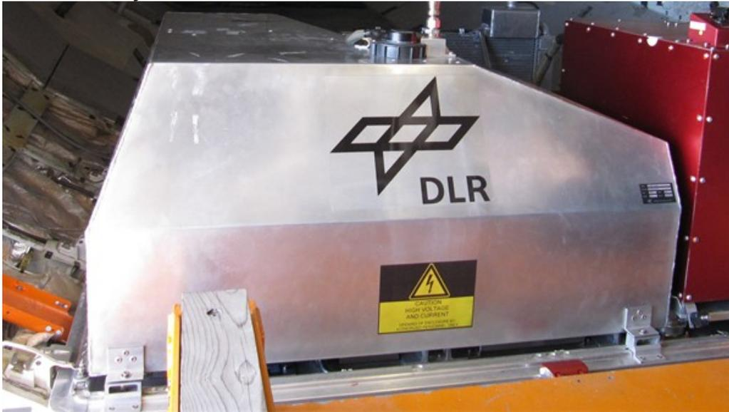
The DLR fuel cell system installed in the ATRA research aircraft.
