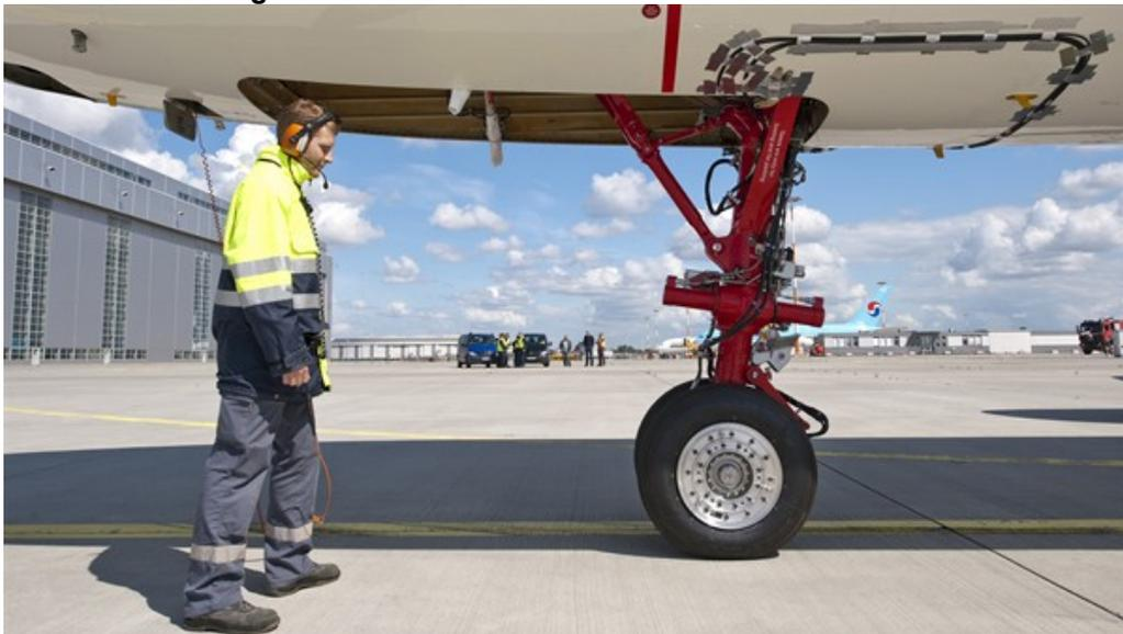
One of the test engineers in front of the electric nose wheel just before the testing began.
