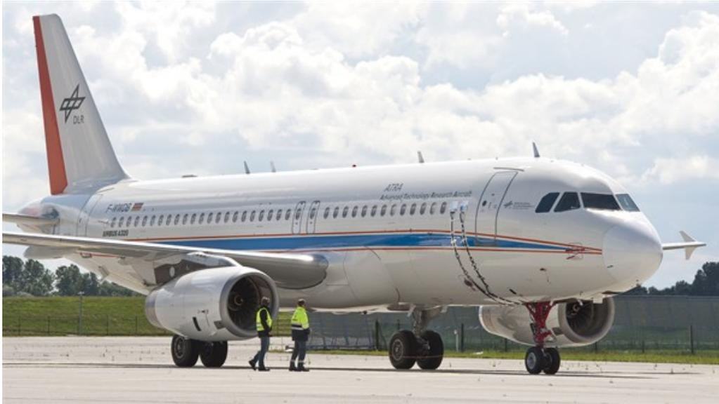
The DLR research aircraft ATRA, equipped with a fuel cell-powered electric nose wheel during testing.
