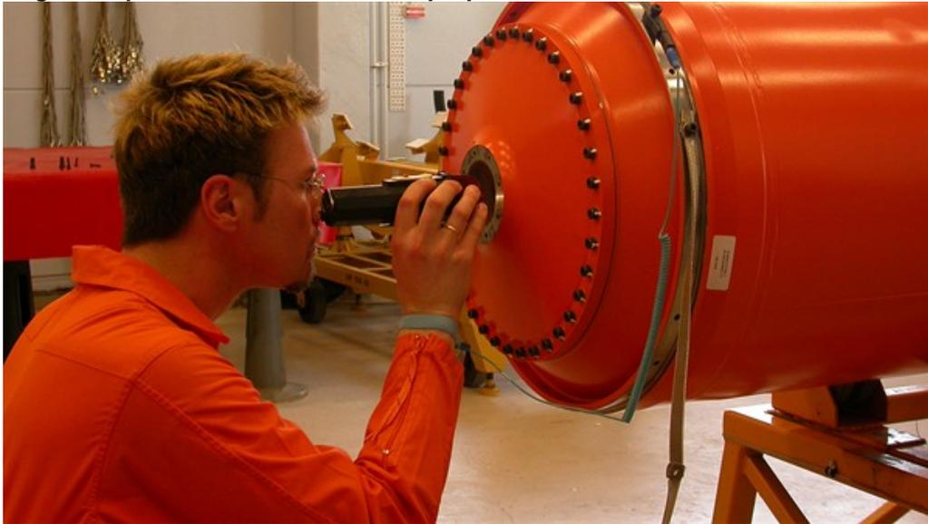
To make sure nothing goes wrong, each propellant assembly of the sounding rockets is visually inspected for possible cracks. In this image Wolfgang Jung inspects the engine of the VSB-30 rocket for the TEXUS 43 mission, launched in May 2006 from Kiruna, in northern Sweden.
