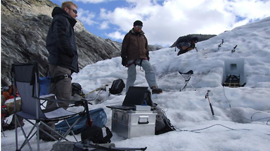
The IceMole is put into operation and, slowly makes its way to the lake underneath the Morteratsch glacier as it melts through various layers of ice.
