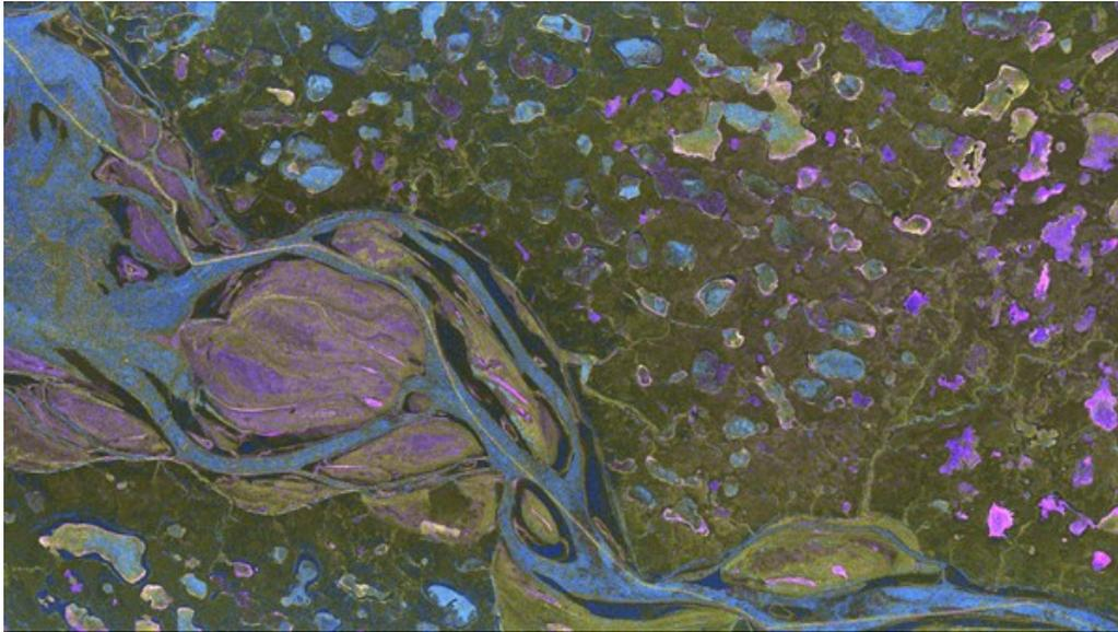
Radar signals from the TerraSAR-X satellite can penetrate the upper layers of snow and ice that cover the Mackenzie River in Canada. The shades of colour enable DLR researchers to draw conclusions about the ice formations and various subsurfaces.
