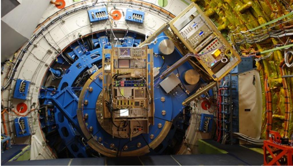
The GREAT far-infrared spectrometer (the vertical structure in the foreground) is mounted to the telescope counterweight flange inside the pressurised cabin. During observations, GREAT rotates  $\pm 20$  degrees from the vertical, while the telescope (invisible on the far side) and its counterweight (seen here in blue at an angle of 45 degrees) move between roughly 25 and 65 degrees from the vertical.
