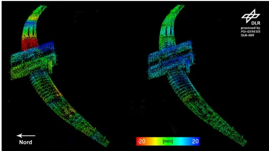
Using TerraSAR X data, Berlin Central Station was measured horizontally and vertically over the course of a year. In the warm season, the steel structure of the building expands; in winter, it contracts again. Based on the coloured dots, the maximum deformation in the course of one year can be seen to be in the millimetre range. The horizontal movement is visible in the left-hand image, and the vertical movement of the station structure is shown in the right-hand image.
