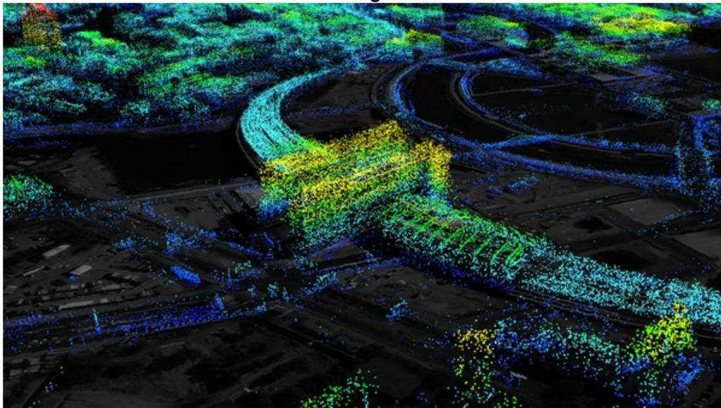
Radar view from above; this data analysis reveals variations in the height of the station and its surroundings. The yellow and red markings in the dot cloud show elevation changes in the millimetre range.
