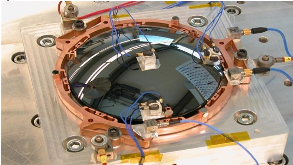
The overall optical design for the near-infrared spectrometer and photometer (NISP) and the lenses of the instrument will be developed and provided by the Max Planck Institute for Extraterrestrial Physics in Garching, near Munich. Shown here is an optical lens holder during the first test.
