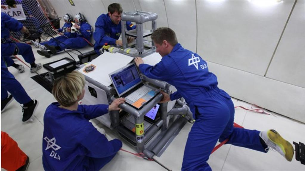
DLR researchers use parabolic flights to test the MASCOT asteroid lander's functions in microgravity. MASCOT is due to separate from the Japanese Hayabusa-2 spacecraft above asteroid 1999 JU 3 and fall to the surface.
