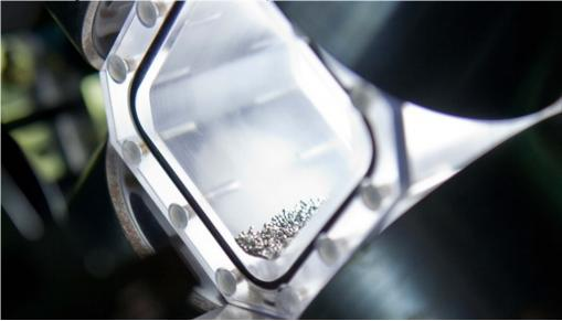
The granulate gases in the MEGraMa-M experiment: When subjected to conditions of microgravity, the spherules float in the brightly lit sample container. The circular electromagnets on the four sides of the container caused the particles to move.
