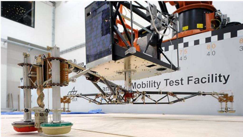
In the test facility for land vehicles LAMA at the DLR Institute of Space Systems in Bremen, scientists are examining how to place a vehicle on another celestial body. Here, a model of the Philae lander, on board Rosetta, which is scheduled to land on comet Churyumov-Gerasimenko in 2014.
