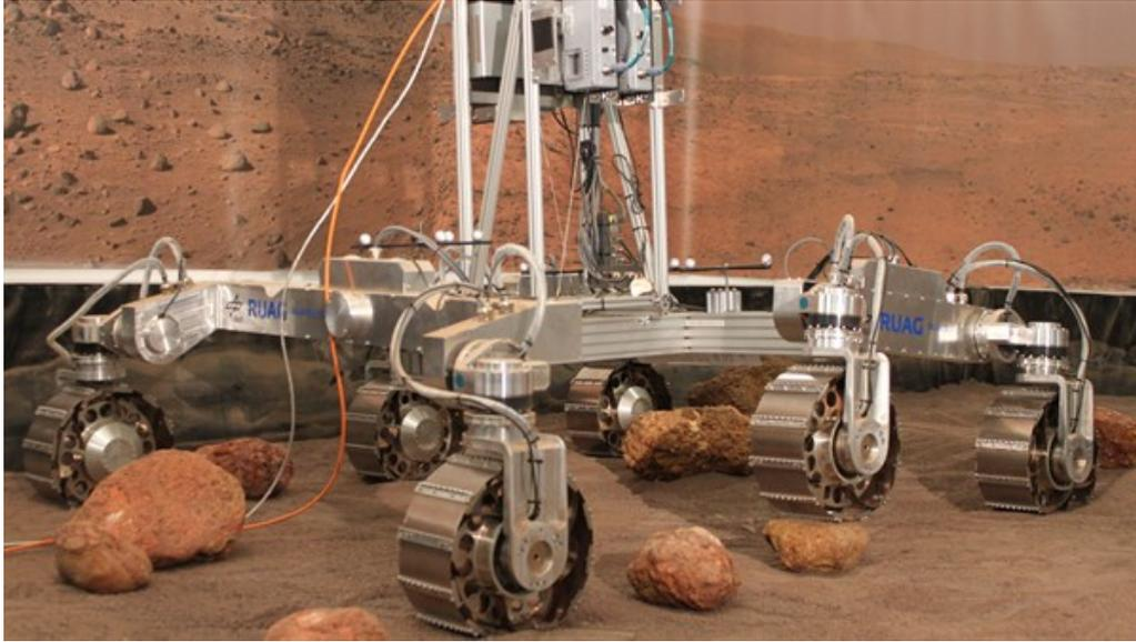
In planetary rover test bed of the DLR Institute of Robotics and Mechatronics in Oberpfaffenhofen, DLR experts test a prototype of the ESA ExoMars rover, which will be launched to Mars in 2018.
