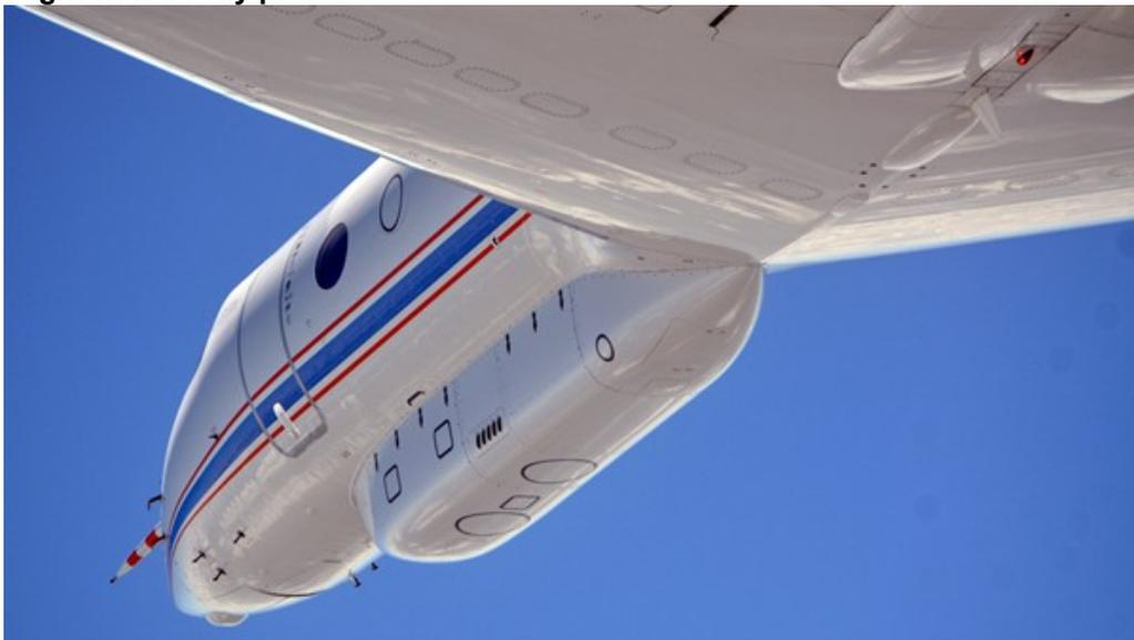
Additional containers for scientific instruments can be attached under the fuselage and under HALO's wings.
