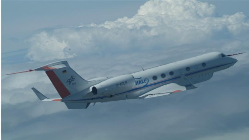
An additional container for scientific instruments is installed underneath the fuselage and wings.
