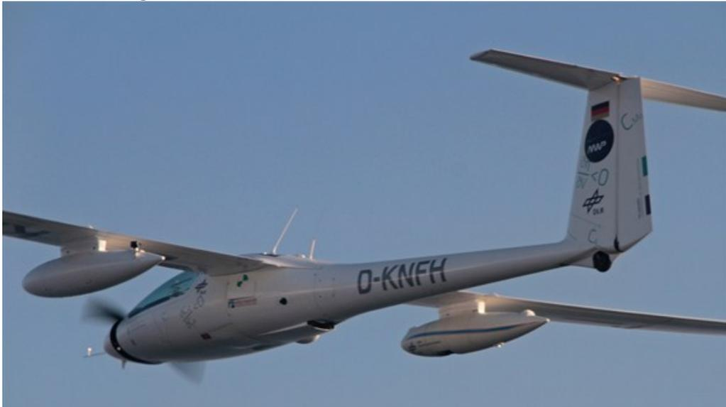
The Stemme S10-VTX glider has a retractable propeller mounted on its nose. The University of Applied Sciences in Aachen contributed the aircraft for the expedition.
