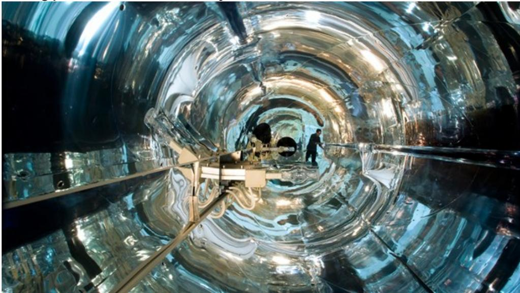
Researchers at the DLR Institute of Solar Research test the receiver performance at the QUARZ Center in Cologne, investigating the percentage of sunlight that the tubes convert into heat. The tests are carried in the ElliRec test stand.
