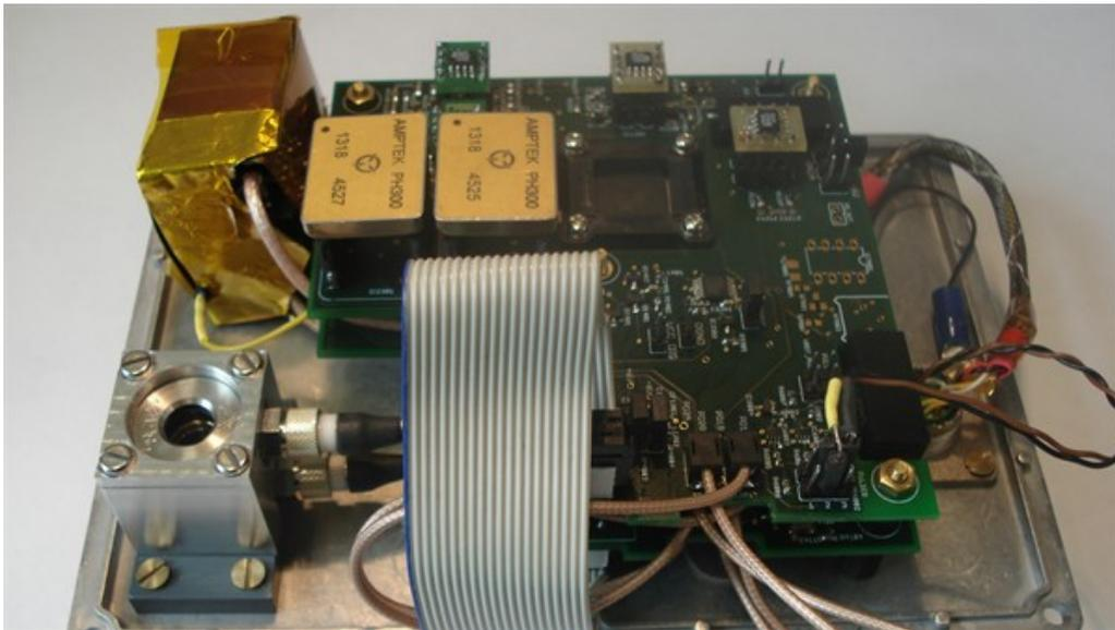
Scientists from the German Aerospace Center (DLR) will use the radiation detector RAMIS to measure the radiation field during the Eu:CROPIS Mission.
