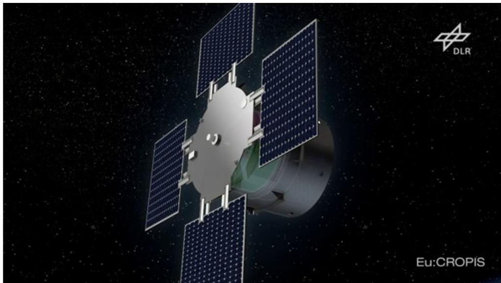
The German Aerospace Center (DLR) Eu:CROPIS satellite is scheduled for launch in 2016. On board will be two greenhouses in which bacteria and algae will convert synthetic urine into fertiliser to promote the growth of tomato plants. Variations in rotational speed around its longitudinal axis will simulate lunar and Martian gravity.
