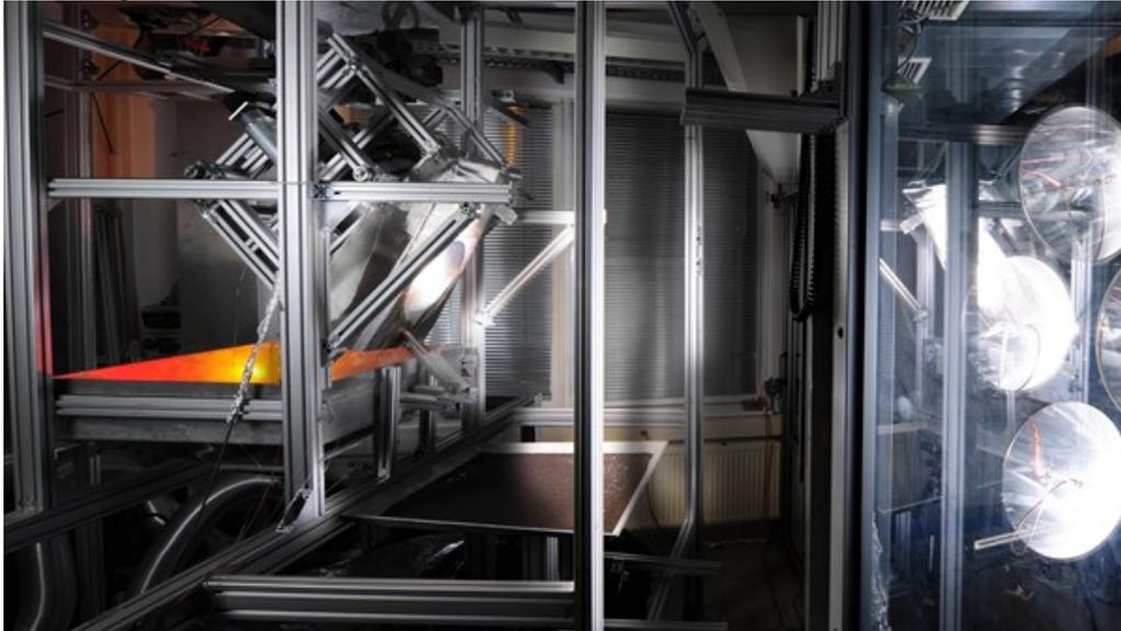
Novel receiver being tested with high-performance radiators at the DLR solar furnace in Cologne.
