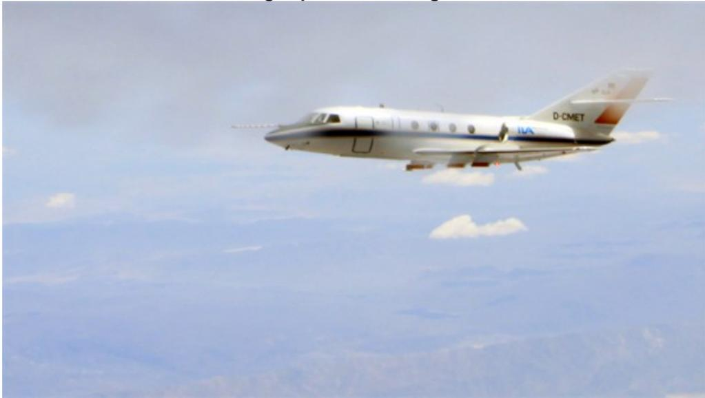
The DLR Falcon flies with its measuring inlets in the upper part of an engine exhaust gas plume.
