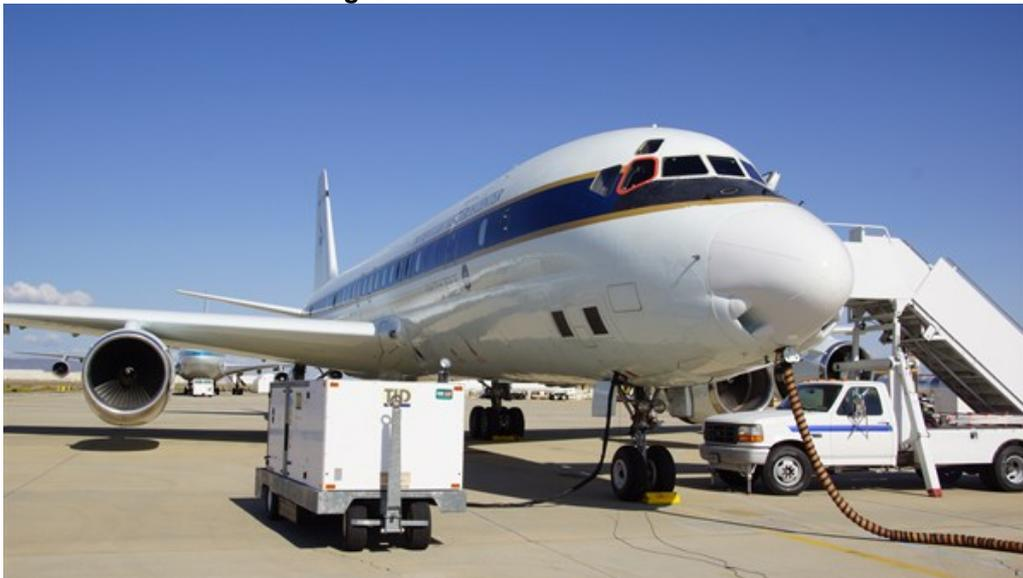
During the research flights, the four CFM56 engines of the DC-8 alternated between regular JP-8 jet fuel and a one-to-one mixture of JP-8 and the biofuel HEFA (Hydroprocessed Esters and Fatty Acids). HEFA is obtained from the oil of Camelina plants.
