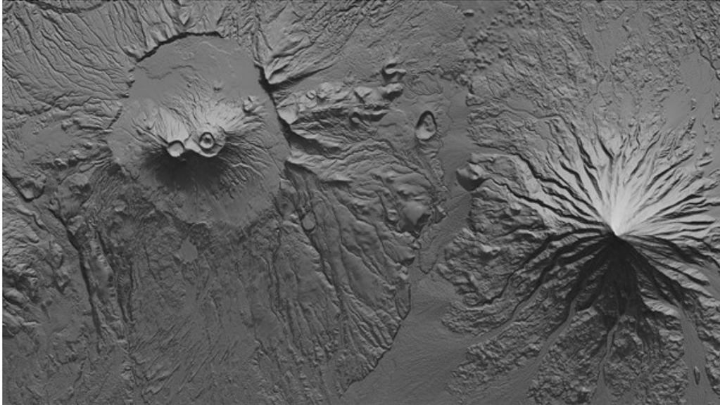
The German Aerospace Center (DLR) is delivering the first final digital elevation models from the TanDEM-X mission for scientific use. Here, a detailed view around the Krasheninnikov Caldera and Kronotsky Volcano is presented as a shaded relief map. Maps of this kind using TanDEM-X data permit analyses of possible lava flow, used to determine endangered areas.
