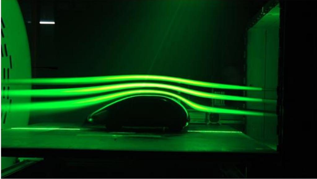
To mark the anniversary, the Göttingen based DLR researchers returned a preserved, smaller original model to the wind tunnel. The images they acquired confirmed the analyses conducted during the 1930s – the airflow clung tightly to the model's contours, causing neither stalls nor turbulence that might slow down the vehicle. The elongated rear, sloping down towards the ground, proved a perfect solution, producing none of the backflow that causes drag in most cars.
