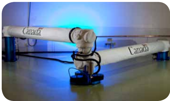
The next generation of large Canadian Space Agency robotic manipulators will feature telescopic booms and will meet the tight packaging and launch constraints of future exploration vehicles, such as Orion.
