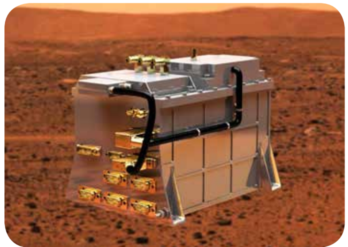
ASI is developing the DREAMS (Dust characterization, Risk assessment and Environment Analyzer on Martian Surface) instrument suite to help characterize Mars landing site environments.
