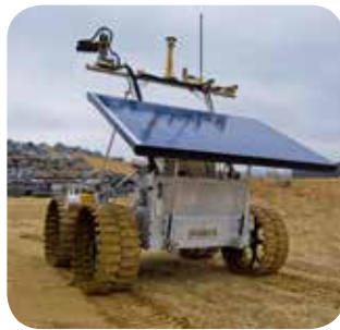
Two rovers demonstrate reliable autonomous mobility software in an analogue environment (K-REX on the left, and Artemis Jr./Canadian Space Agency).
