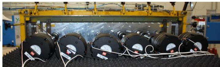
Figure 9: FDF test rig for high-speed testing of liners (left) and ZML-liner setup at FDF test section (right).
