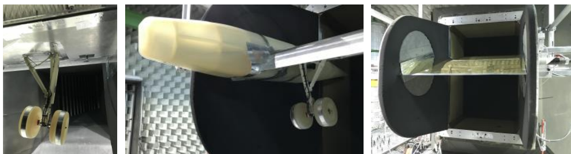
Figure 6: ARTEM test configurations in AWB . (© DLR, 2019)
