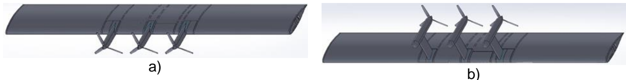
Figure 12: DEP wing: a) configuration with three tractor propeller units, b) configuration with three pusher propeller units. (©PVS, 2019)
