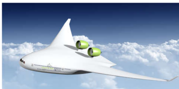
Figure 1: Left: A possible candidate for 2035 air transport: ONERAs NOVA concept with semi-buried engine (© ONERA, 2015). Right: Initial layout of a blended wing body anticipated for 2050 operation, equipped with generic UHBR engines mounted on pylons on the top of the centerbody (© University RomaTre, 2018).
