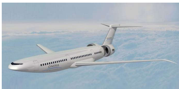
Figure 1: Left: A possible candidate for 2035 air transport: ONERAs NOVA concept with semi-buried engine (© ONERA, 2015). Right: Initial layout of a blended wing body anticipated for 2050 operation, equipped with generic UHBR engines mounted on pylons on the top of the centerbody (© University RomaTre, 2018).
