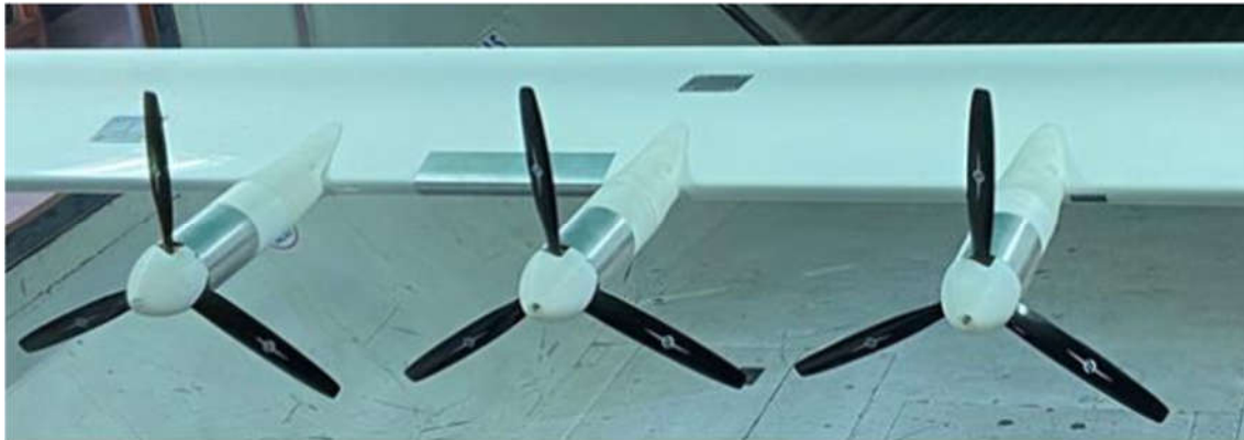
Figure 13: "Tractor" (or puller) configuration of the three propellers (© INCAS, 2020).
