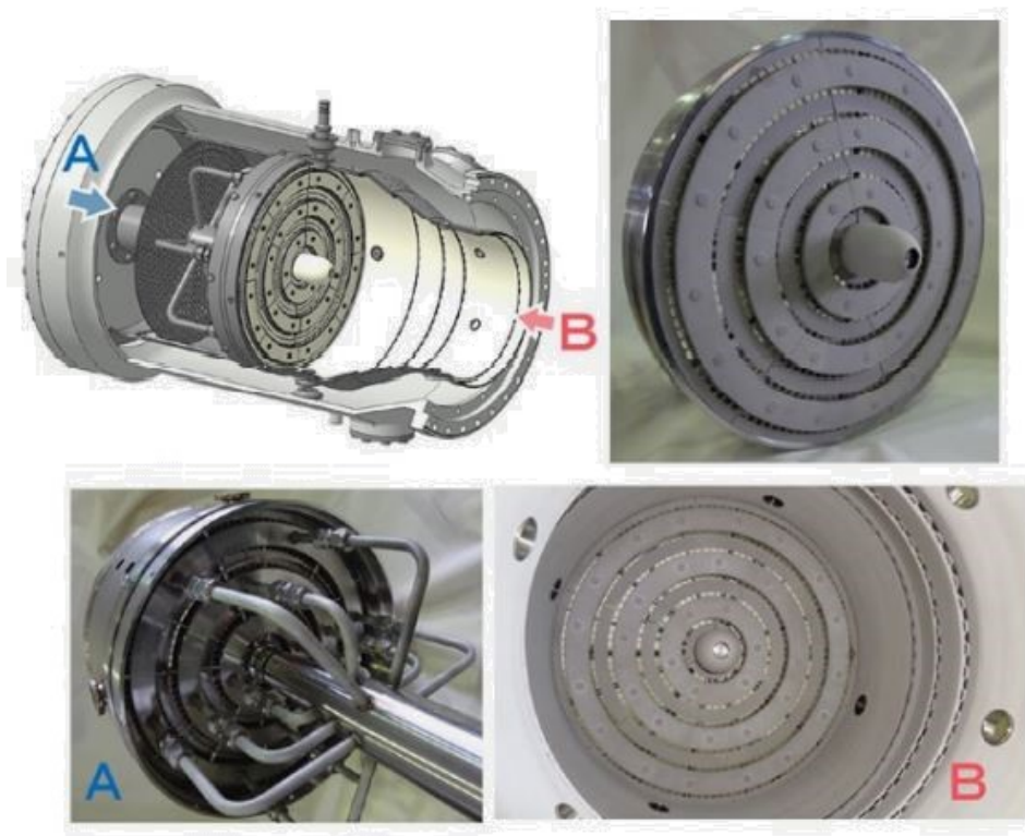
Figure 25: Design of a Micro-Mix combustion burner [11]
