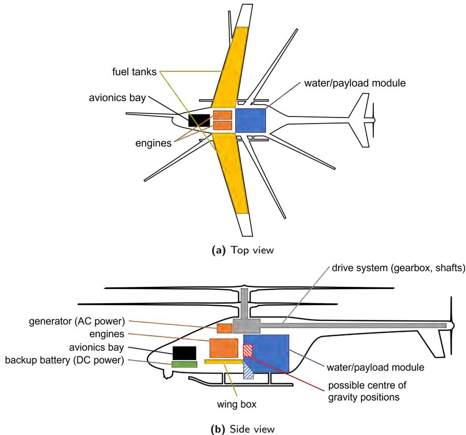
**Figure 3.3:** Internal component Layout of FireWasp
