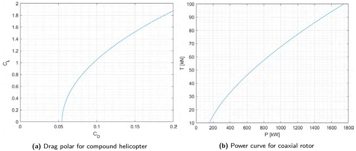
**Figure 3.6:** Relations used during performance calculations
