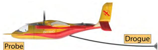
Figure 5.6: Drogue-and-probe concept for aerial refueling and maximizing firefighting time
