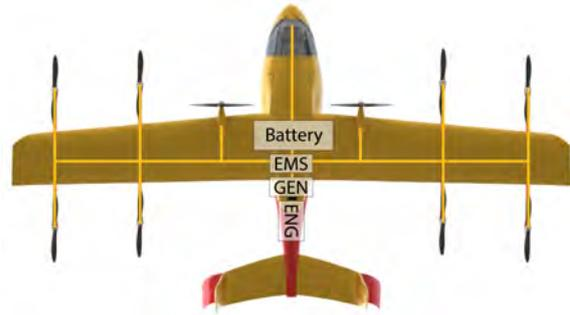
Figure 4.8: Illustration of the hybrid energy storage system
