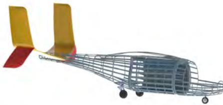
Figure 4.14: Structural concept of fuselage with module installed
