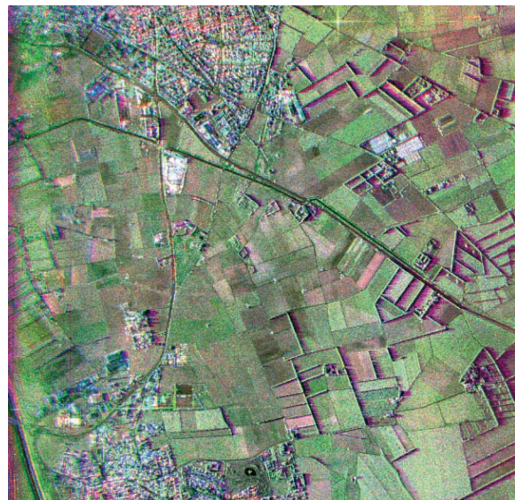
Figure 2.96 Colour composite of three SAR images with different bistatic angles, showing the good differentiation of surface features.
