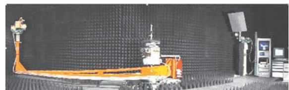
Figure 2.157 Monostatic and bistatic RCS measurement facility with the reflection measurement system on the right. The test object is located on the rotator in the center, and the transmitter antenna is mounted on the arm.
