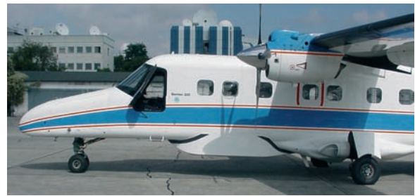
Figure 2.144 P-band antenna with the wind deflector mounted under the fuselage of DLR's Dornier Do 228.
