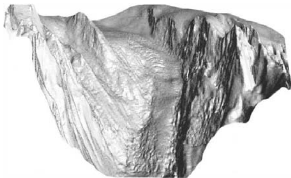
Figure 2.63 Digital Elevation Model of the Engabreen Glacier in Svartisen, Norway acquired in X-band single-pass SAR interferometry. The height varies by approx. 1500 meters in this sub-image of ca. 2 km x 2 km.
