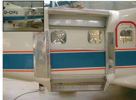
Figure 2.85 New F-SAR antenna mount attached to the right-hand side of the aircraft behind the wing allowing 7 antennas to be integrated.
