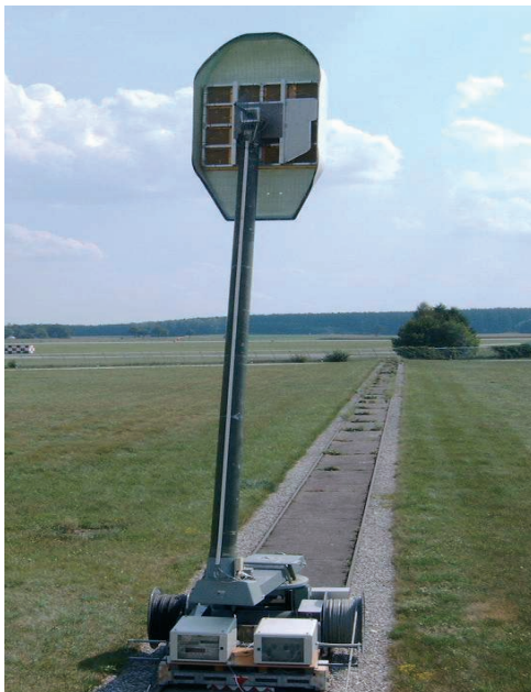
Figure 2.151 DLR's airborne P-band SAR antenna mounted with its wind deflector on the antenna measurement facility AMA.
