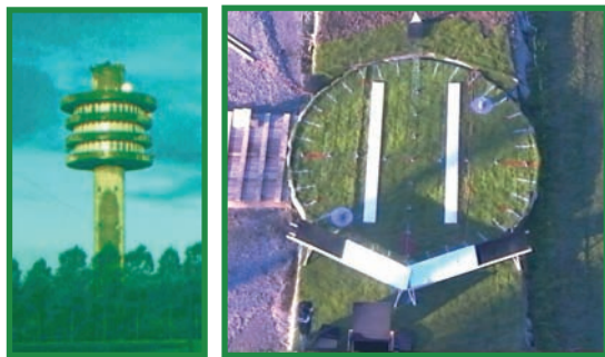
Figure 2.108 Photograph of the tower-turntable arrangement at the Meppen proving ground. Left: The tower with different platforms at heights between 30 m and 50 m. Right: the turntable about 9 m in diameter.
