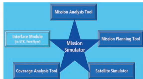
Figure 2.42 Modular design of the mission simulator with the four core modules: mission analysis tool, mission planning tool, satellite simulator, Coverage Analysis Tool (CAT) and interfaces to COTS software products.
