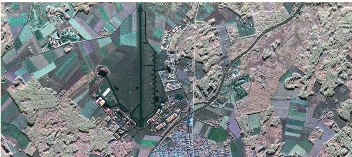
Figure 2.57 Fully polarimetric E-SAR image of Oberpfaffenhofen, incl. DLR facilities in image center; composite obtained from 2 dual-polarized data takes in C-band (HH-green, HV-red, VV-blue).
