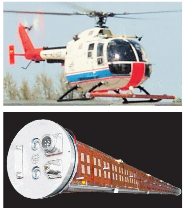
Figure 2.98 Top: Antenna system attached to the skids of the helicopter. Bottom: SIREV antenna with 56 receiving subarrays.
