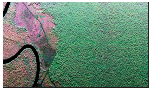
Figure 2.67 P/X/L-band polarimetric intensity image of the Mawas test site with a disturbed burned forest area (red) and a natural tropical forest (green). This is a geocoded image with a spatial resolution of 2 m x 2 m. Colour Composite: red - P-band, (HH+HV+VV)/3 ; green - X-band, VV ; blue - L-band, (HH+HV+VV)/3 .
