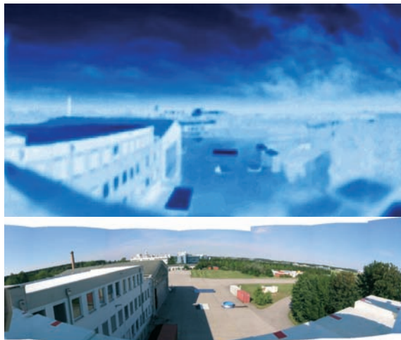
Figure 2.164 Top: line-scanner image of a complex scene at 90 GHz taken from the roof of the Institute; bottom: a corresponding panoramic photograph.
