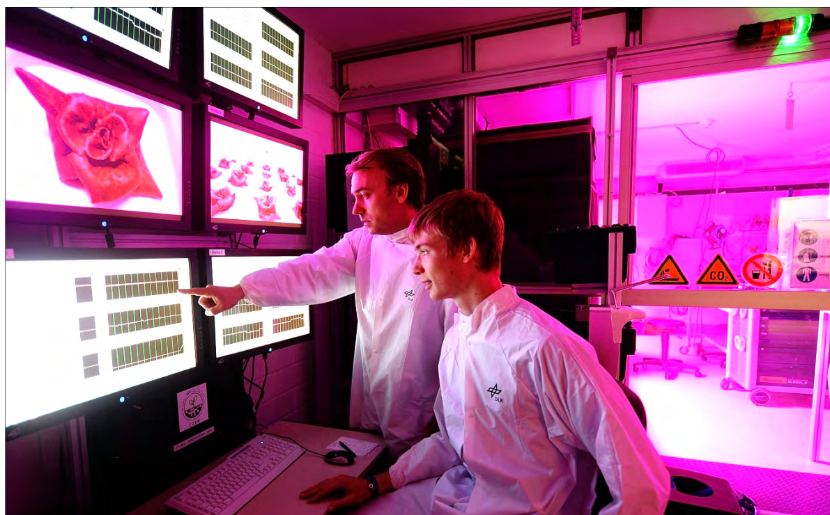
Figure 13: Main control station of the closed-loop test facility within the EDEN Laboratory. All sensors data and visual monitoring feeds are linked to this control station in order to monitor plant growth, but also to test remote control technologies.
