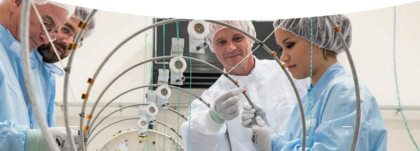
Integration of deployable helix antenna for AISat-1
