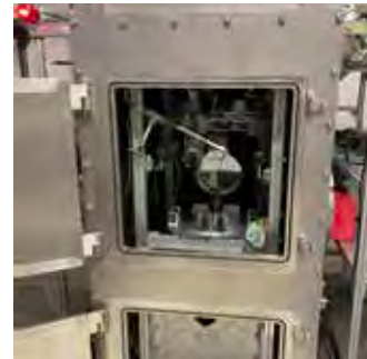
Thermal vacuum chamber which will be used for the LUWEX water extraction and capture experiment
